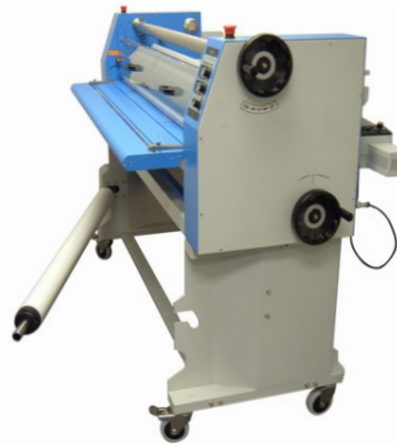
Motorized rear rewind for roll-to-roll applications
